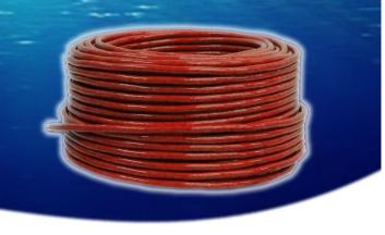
Our underwater communication and data cable is designed for the commercial diving industry. The 1.8mm (0.070 in) wall thickness Pressure Extruded Polyurethane jacket is extremely resistant. The cable integrates high tensile Aramid Fiber (KEVLAR™) that extend the breaking load to 22 kN (5000 lbf)! Our CDC cable has all conductors required to operate all diving communicators OR AXSUB® AxDEPTH depth sensor.
