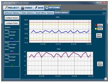
The default page contains only one basic chart. This chart can be used to display any kind of data from an Analox sensor. Also, the same chart can display data from multiple sensors at the same time. Clicking the <u>Configure Charts</u> button allows the user to make changes to the charts. Names can be given to the charts, high and low alarms can be set and new charts can be added by clicking the <u>Add Charts</u> button.
