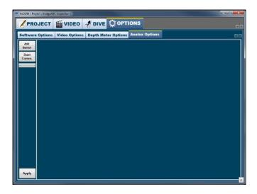
New sensors can be added by clicking the <u>Add Sensor</u> button. Serial numbers of the devices can then be entered in the corresponding boxes to allow communication. Names can be given to the sensors with the sole purpose of making it easier to remember which device is what. Display configuration about the line color on the chart and the chart selection can also be chosen here. Finally, devices can be deleted by clicking the Del. button.
